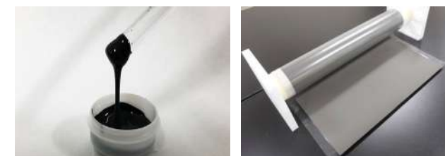
Newly developed magnetic materials (Left) Paste type (Right) Film type
